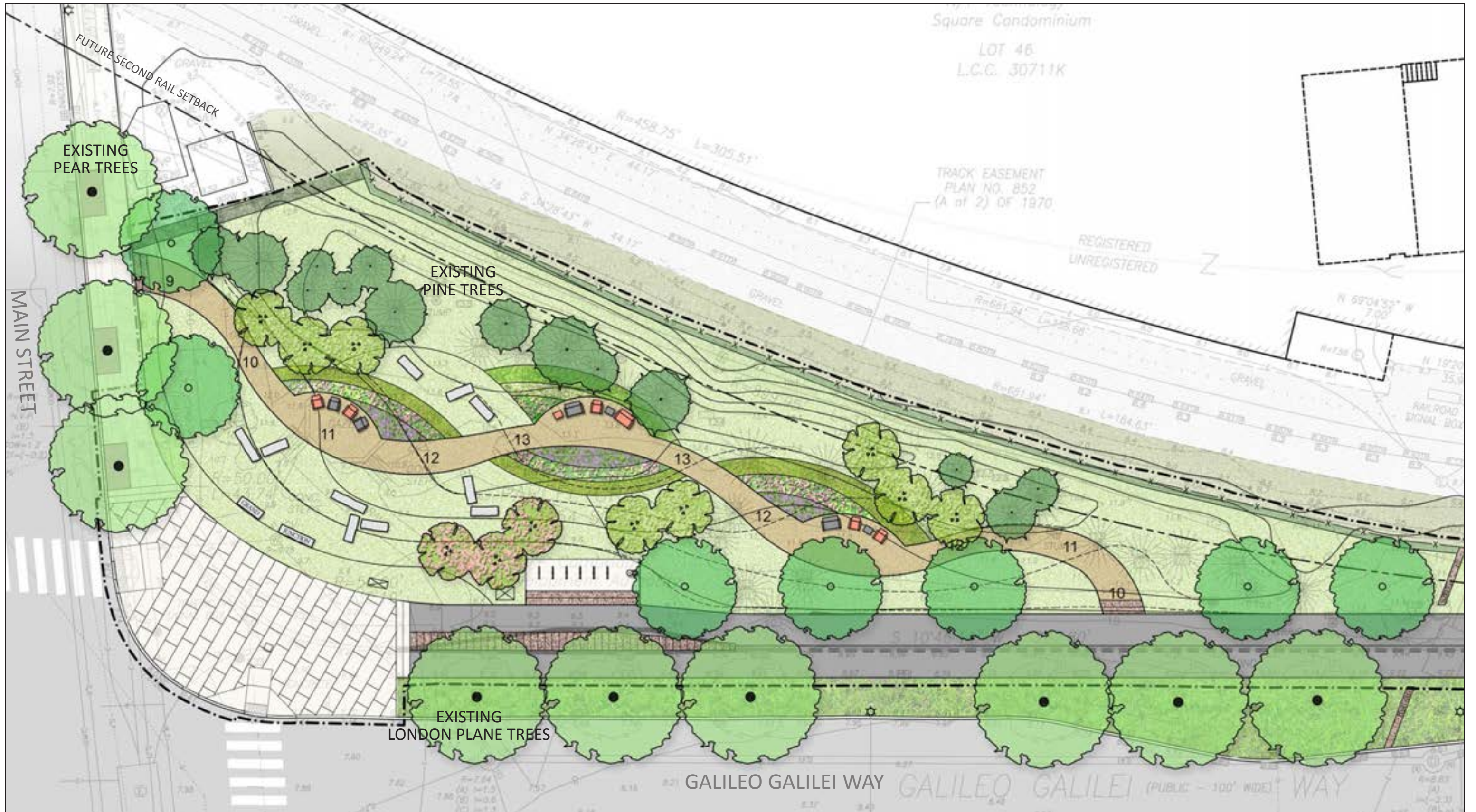
SITE PLAN: OPTION 1A - Long Path with Expanded Granite Seat Blocks and No Children's Play
