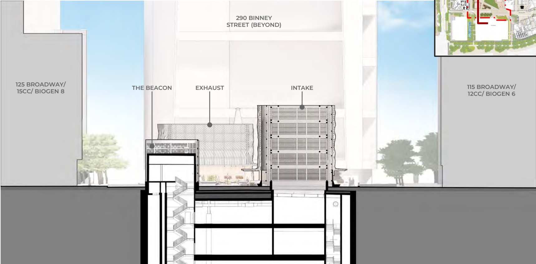
Looking North - Through Beacon and Intake
