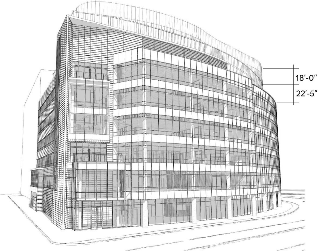
ALTERNATE 18' ROOF SCREEN
