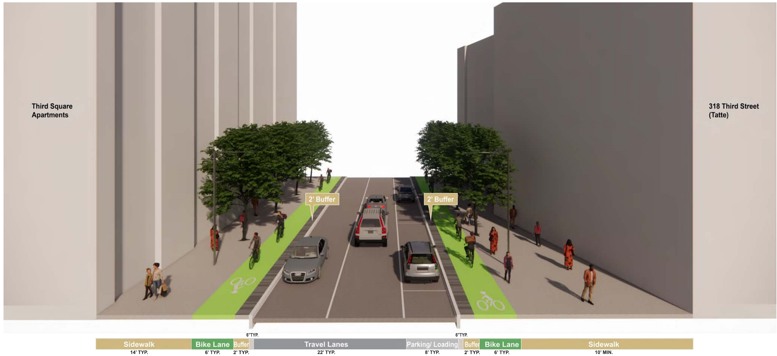
Figure 5-10 Third Street Cross Section Between Athenaeum Street and Linskey Way - Two-Lane Approach
