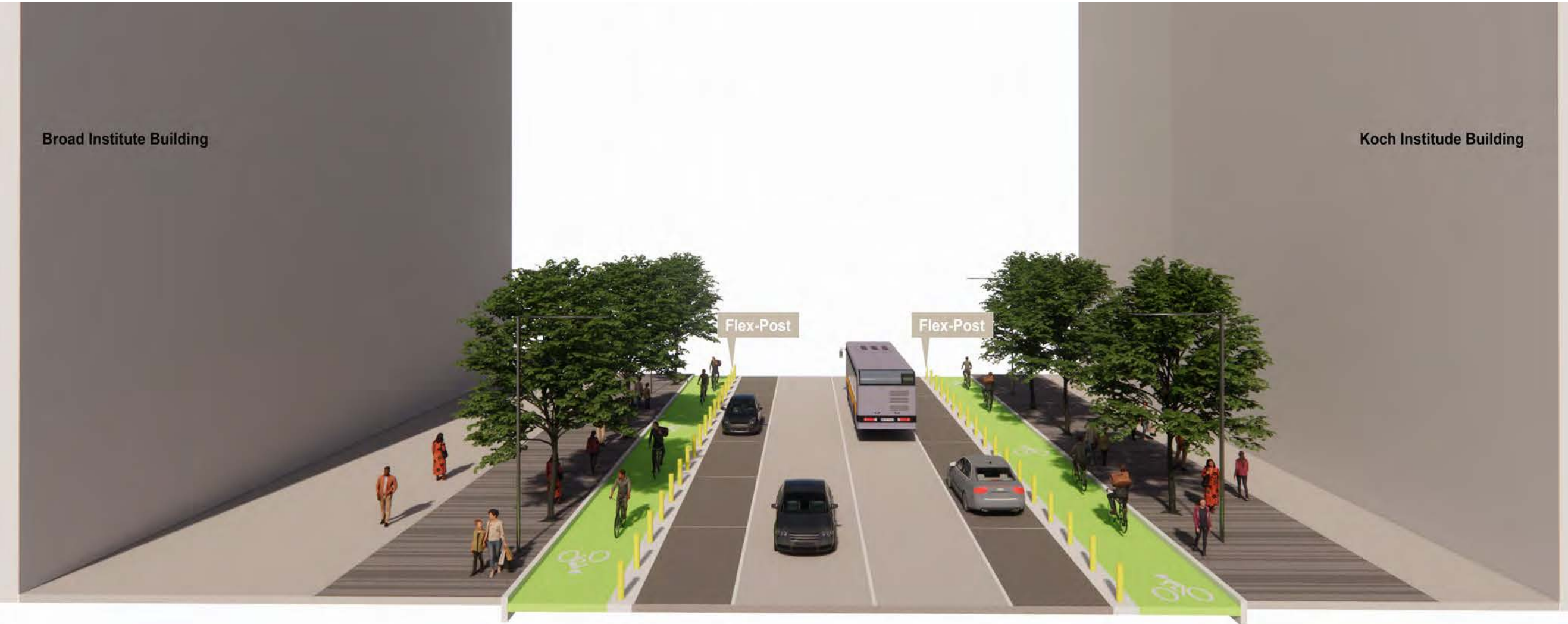
Figure 5-19 Main Street Section West of Ames Street
